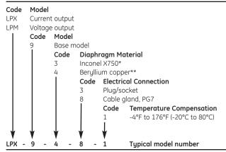
\* Available pressure ranges from 0.4 inH<sub>2</sub>O to 15 psi \*\* Available pressure ranges from 0.04 to 0.8 inH<sub>2</sub>O
